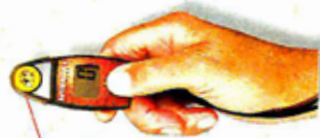
HOUSING ROTATES TO PROTECT IMPELLER
