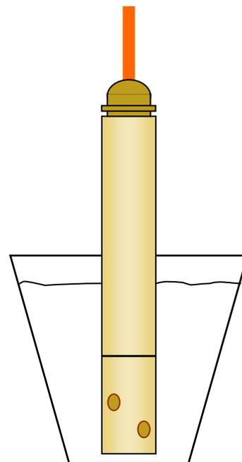
Before starting the calibration, the probe should have the water's temperature, which can be checked by putting the device in **MULTIMETRE** mode. Ensure that the temperature remains stable. Once all parameters meet these conditions, the calibration can be launched. Only few seconds are necessary.
