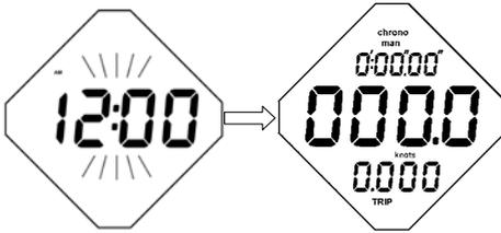
The SPEEDWATCH is now in Manual Mode; it will only receive data from the transmitter when the CHRONO button is pressed and the impeller is rotating. The default speed is knots, which can be changed to mph, km/h, or m/s.
